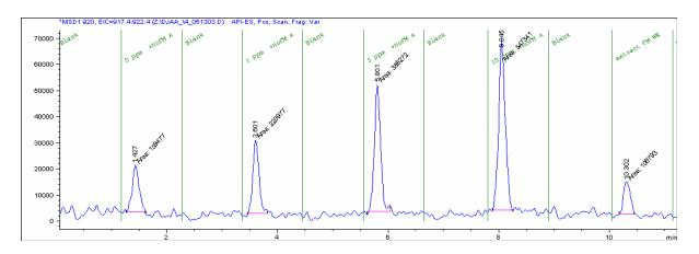
ESI-MS Analysis of an extracted ion plot compares the area under the curve at a key frequency which corresponds to the processing aid component only to determine processing aid level.
