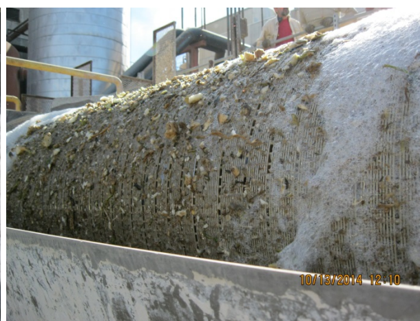
Figure 5: Rotary Screen Operation
