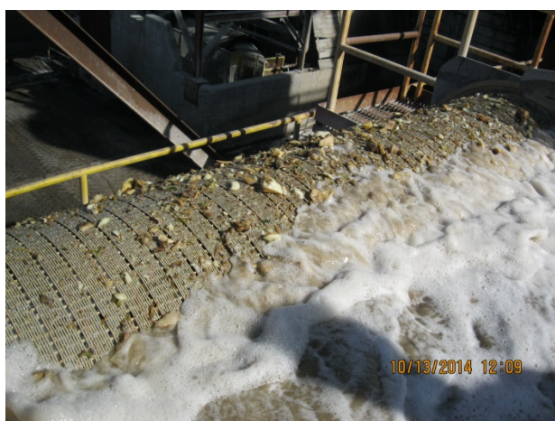
Figure 4: Rotary Screen Operation
